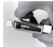
3. Grasping adjustment pin, compress spring and place adjustment bushing assembly over round pin.
