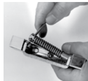
2. Slip bushing over hexagon pin on mounted hinge; then insert adjustment pin into adjustment bushing assembly.
