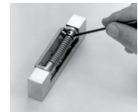
4. Adjust tension; then insert stop pin in hole of adjustment bushing assembly.
